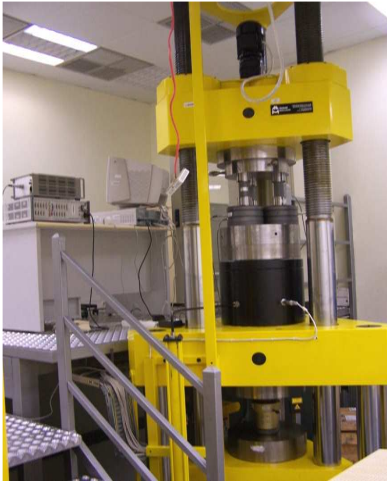
Figure 28: TUBITAK UME 3 MN Build-up force st. machine
